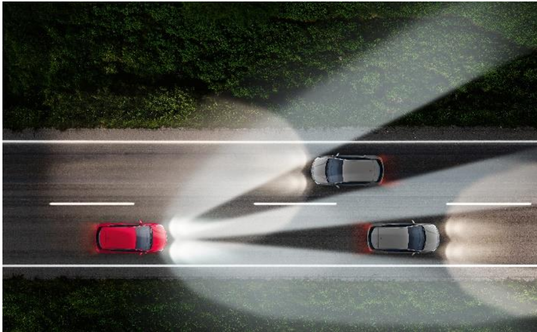
Figure 4: Functional illustration of the adaptive high beam (Source: Opel Media/Stellantis)
