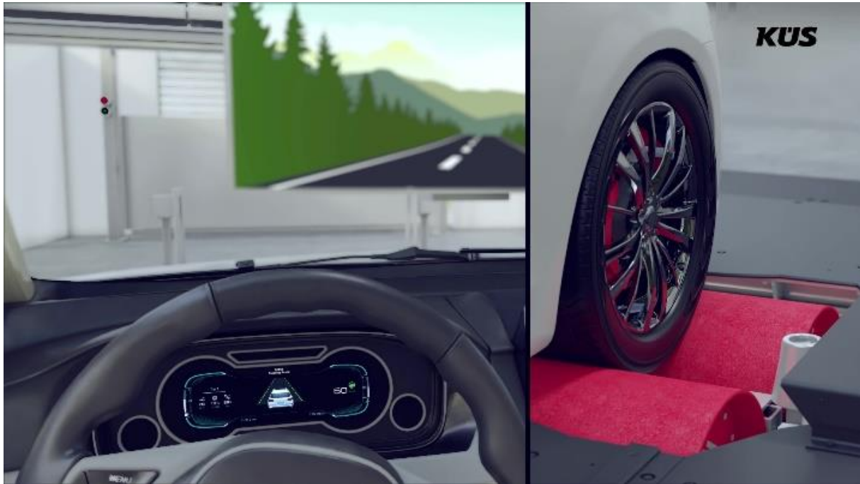
Figure 6: Impact testing of LKA in KÜS DRIVE (source: KÜS)
