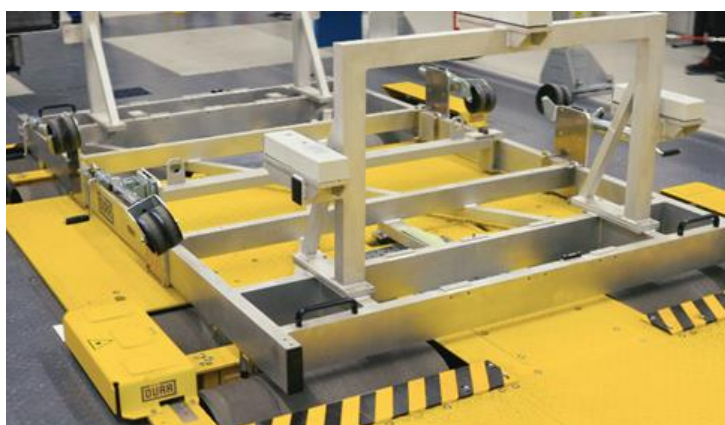
Figure 5: Calibration gauge for KÜS DRIVE on the lifting bars of the SFT (Source: KÜS)
