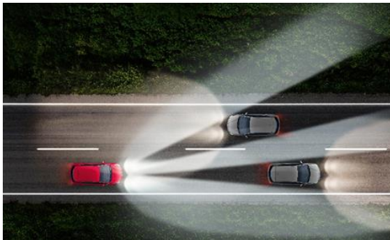
Figure 12: Functional representation of the adaptive high beam (Source: Opel Media/Stellantis)
