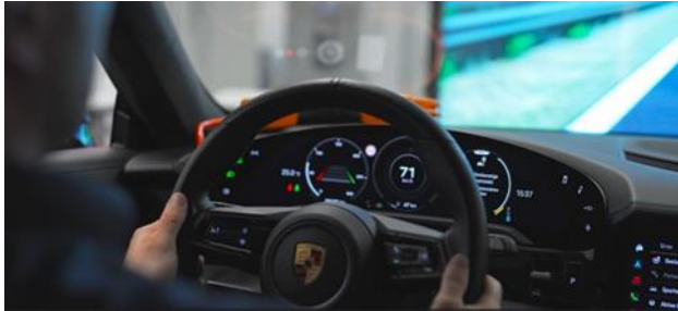
Figure 14: LDW impact testing in KÜS DRIVE (Source: KÜS)
