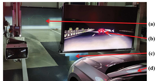
FIGURE 6. KÜS DRIVE during a test run [41]: (a) Laser projection of the target vehicle on the projection wall lowered in working position, (b) Screen extended in front of the VUT for front camera stimulation. The simulated target vehicle is visible as a preceding car, (c) The radar target simulator with absorbers (only partly visible from this angle). The stimulator is extended exactly in front of the VUT radar, (d) VUT.
